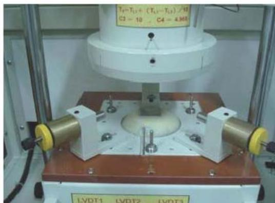
Fig. 1. The core part of the TIM thermal resistance and thermal conductivity measurement apparatus (LW-9389)
